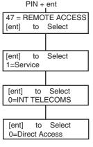
The **1=Service** option enables the user to control the access mode of the remote servicing package. There are 4 communication devices available.
