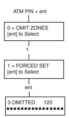
When enabled, the **Forced Set** option allows the user to automatically omit zones, eligible for omission, which are open when the system setting routine is started. Zones omitted in this way remain omitted for one set period only.
