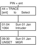
This option provides a record of the most recent alarm activation. The Trace option records the details of the setting and unsetting of the system immediately before and after the alarm activation and the first 5 events occurring during the alarm activation. This information is maintained in the trace until the next alarm activation. On entering the option pressing the **A** and **B** keys steps through each of the 7 trace entries.
